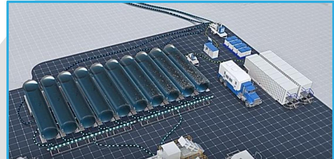
60,000 bpd Self Contained Operation pulling directly off Disposal Site Pipeline, Pumping back into Pipeline for Frac Reuse Eliminating need for Raw Fluid Storage
